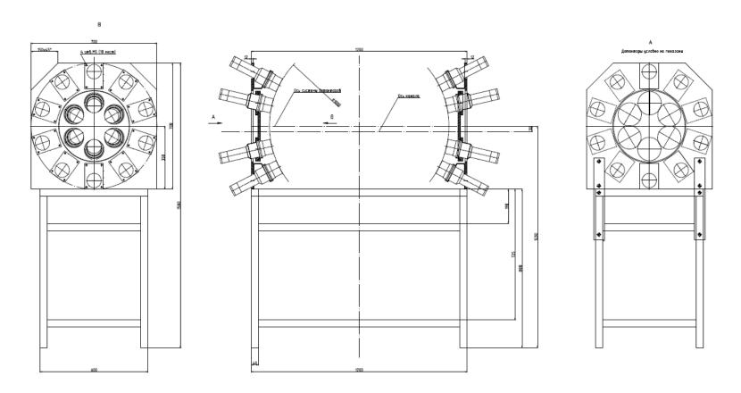
For this new facility new Twin chamber was developed and tested. Thanks to position sensitivity of the chamber the cosine of angle between Fission axis and PFN can be measured with accuracy better than 0.02
