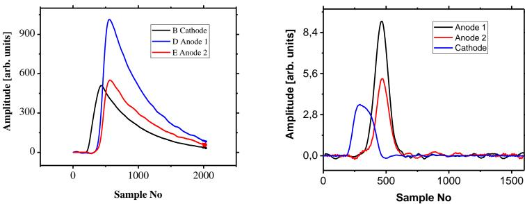
In our approach we have oversampled FF signals. The oversampling we used to increase the effective number of bits (ENOB) improving the signal representation. In practice the increase of ENOB realized automatically when signal passed through second order low pass filter:
