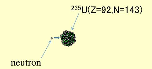
JQMD: JAERI Quantum Molecular Dynamics = a semiclassical molecular dynamics for nuclear reactions (mean field + NN collision)
