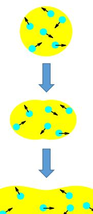
Nuclear shape evolution is driven by random kicks by nucleons in thermal equilibrium (microscopic d.o.f.) given to the nuclear surface (macroscopic d.o.f) from inside the surface
