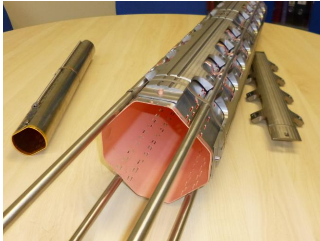
Beam screen prototype for cryogenic test
