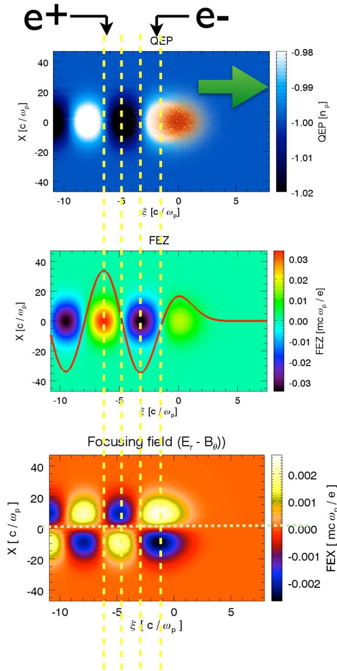
Beam Parameters:  $\sigma_r = 200 \mu\text{m} = 9.4 k_p^{-1}$   $\sigma_z = 30 \mu\text{m} = 1.414 k_p^{-1}$
