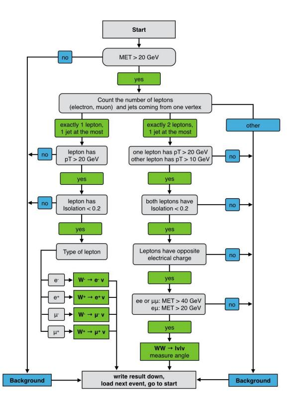
Figure 4: Flowchart for analysis in the ATLAS W path
