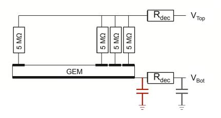
Cable between a Power Supply and bottom decoupling resistor
