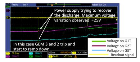
• Another case where we induced the discharge by increasing the voltage on the top of GEM 2
