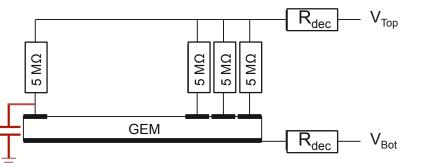
• Extra capacitance (e.g. cable) between the top loading resistor and the top GEM electrode may influence the propagation behavior
