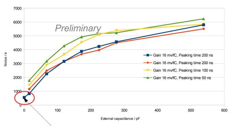
External capacitance decoupled → minimum noise: 560 e
