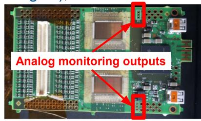
For fast signals (ramp, pulse), ADC is to slow
