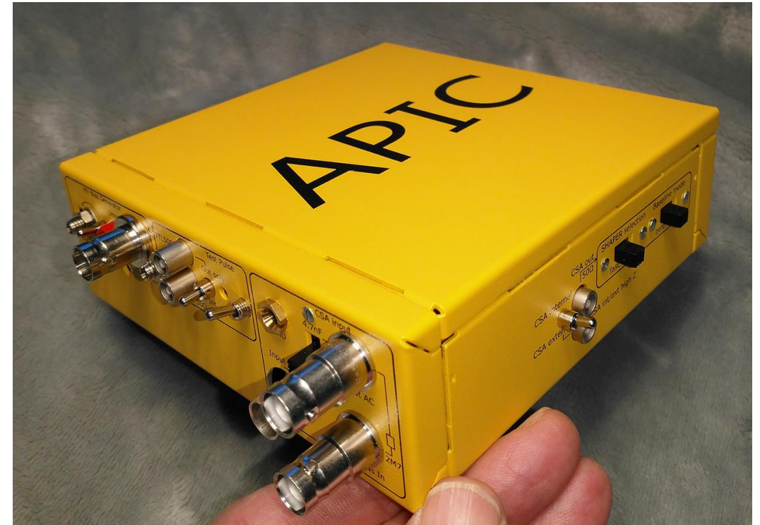
Bias HV, Test and Detector Input - CSA- and shaper selector
