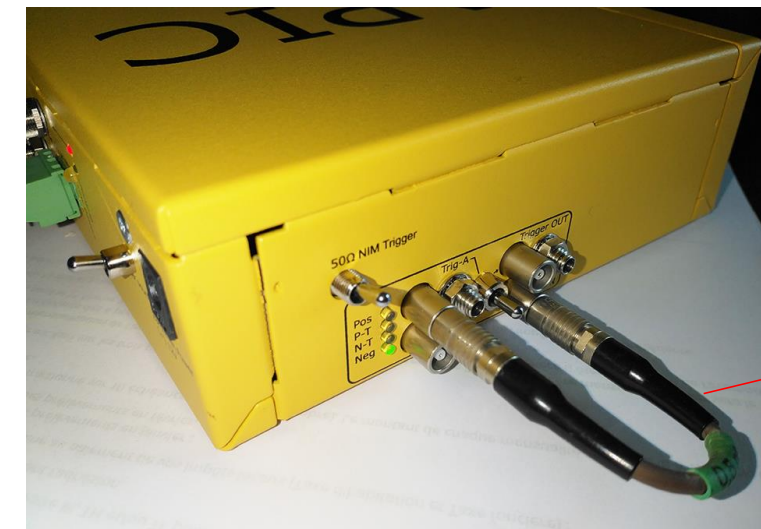
0.5 ns coax cable from A to-NIM trigger input
