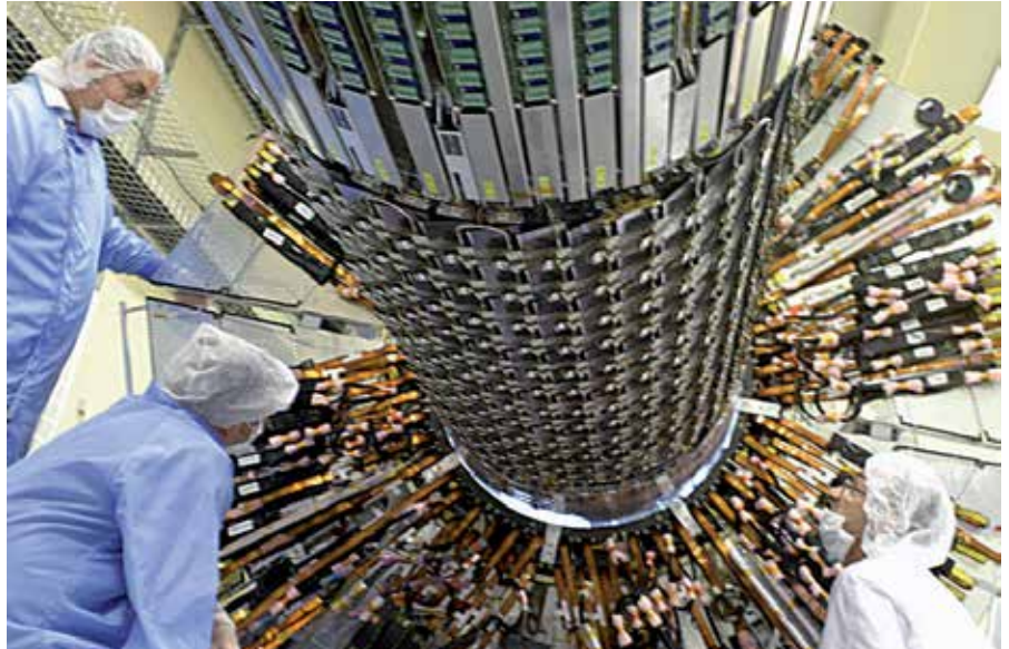
Silicon pixel detector technology being readied for CERN's ATLAS experiment.
