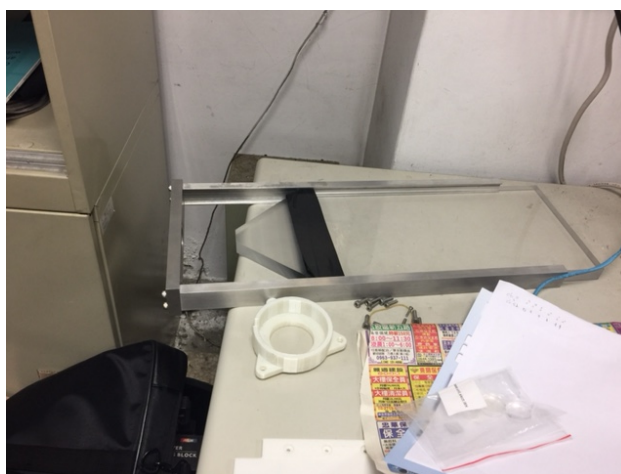
Fig. b, Showing the part of the frame to hold the scintillator.
