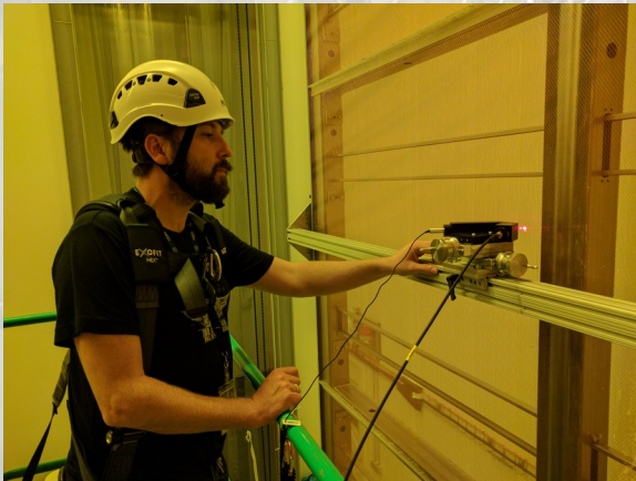
Wire tension measurement and visual inspection
