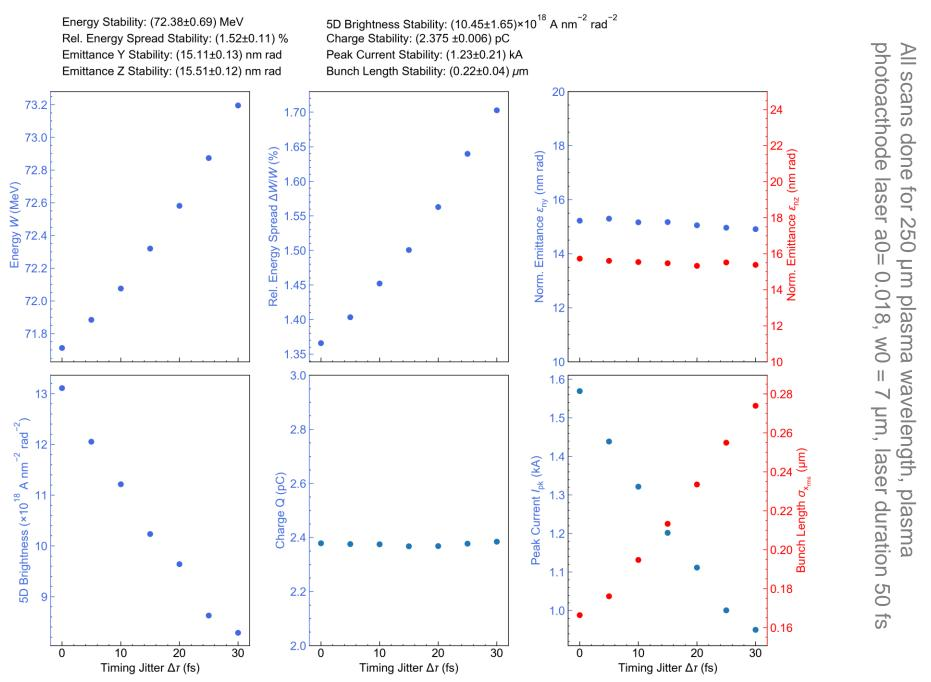
Preliminary FEL simulations, including extraction, capture, transport, conditioning: hard x-ray-FEL with ultrahigh gain (10 m undulator):
