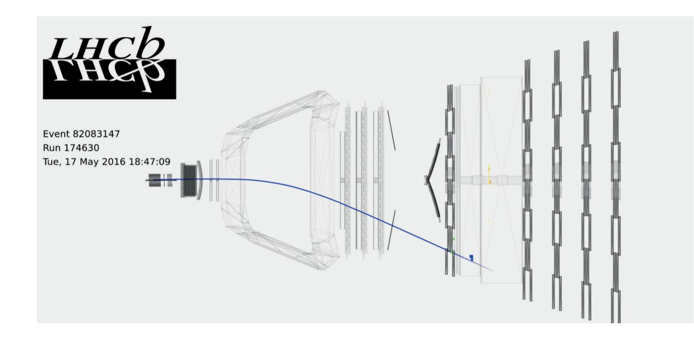
These events are identified by a single low momentum and low  $p_T$  electron track, with no other activity in the detector. A **large background** comes from soft inelastic nuclear interactions. These can be subtracted due to their **charge symmetry** by reconstructing **both single electron and single positron** events and taking the difference in the  $e^-$  and  $e^+$  yields as the signal yield.
