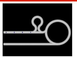
Delay loops create drive beam bunch-structure
