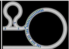
Low energy high current drive beam -> high energy low current main beam
