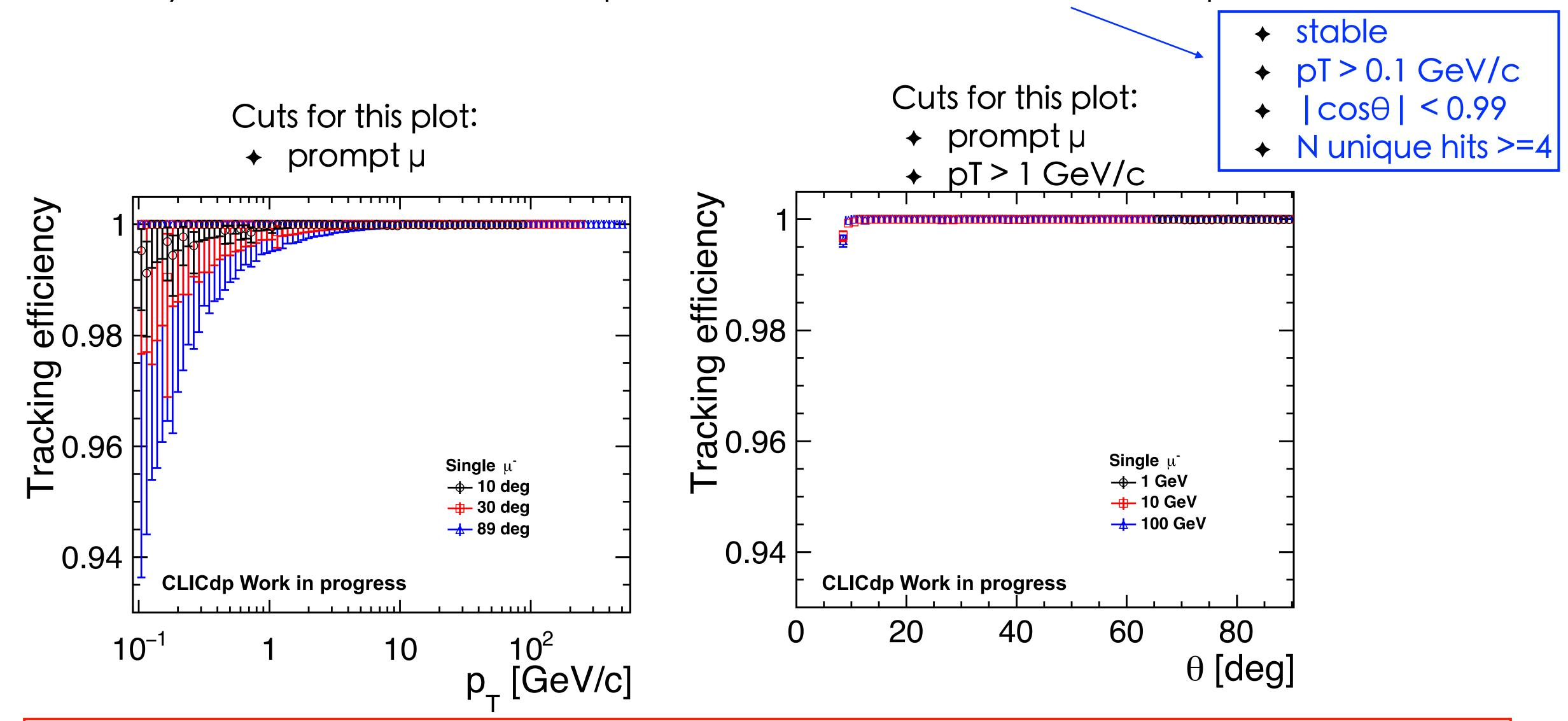
Efficiency = 100% for single muons above 1GeV/c and for the full acceptance above 10deg
