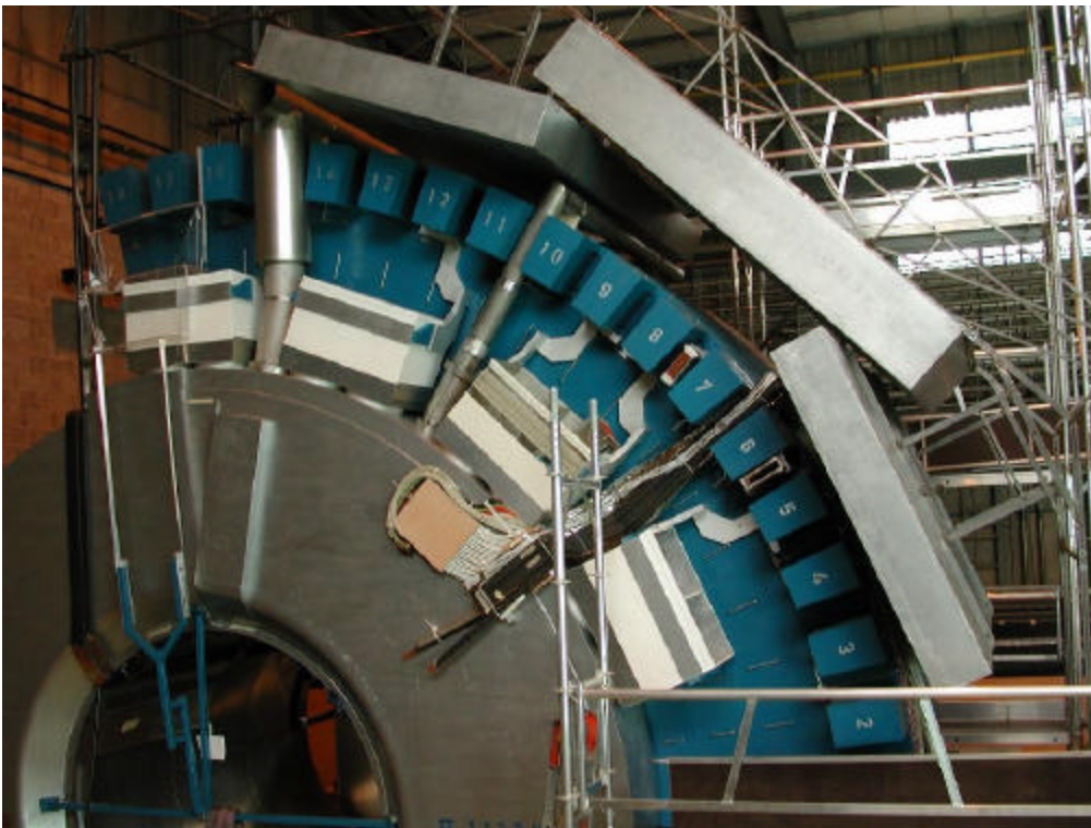
Full-scale mock-up of the ID, LAr barrel, tile calorimeter and inner barrel muon chambers to study the services routing
