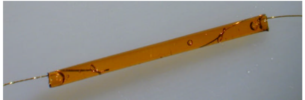
Polyimide-encapsulated epoxy joint (the new wire joint retained after the first milestone end of March, and being pursued now for final decision in May)
