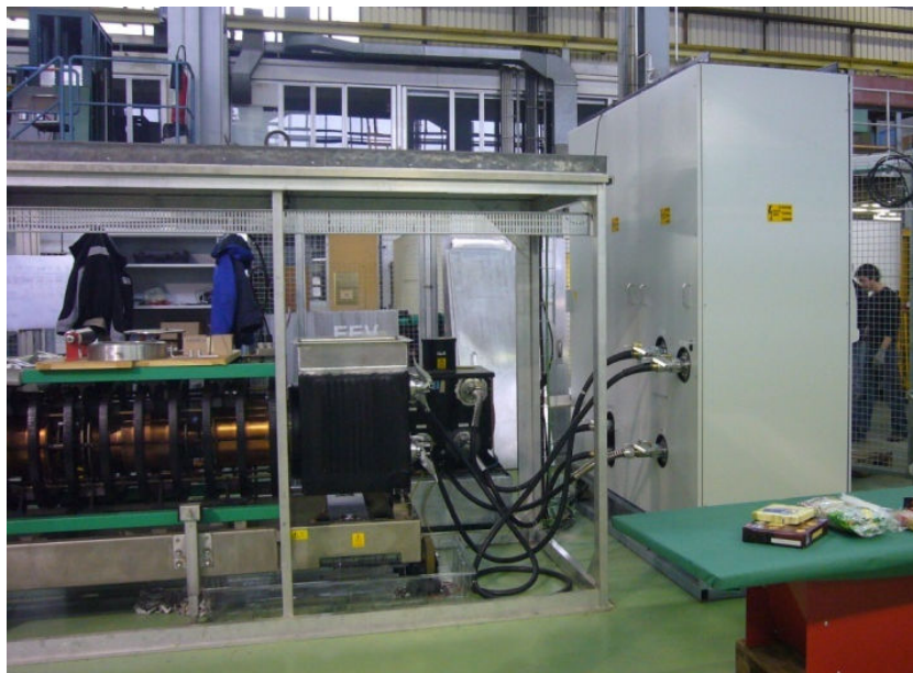
352 MHz Klystron pulsed mode test set-up : 1.3 MW achieved.
