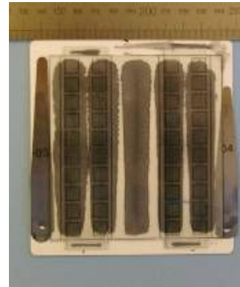
Glue pattern trials (left - on test board , right – on test bus cable)
