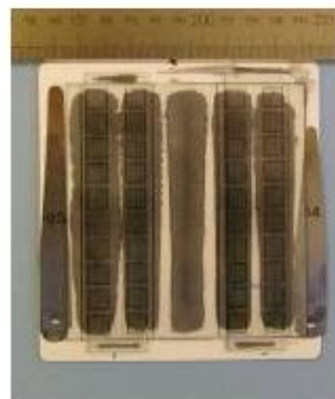
Glue pattern trials (left - on test board , right – on test bus cable)
