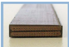
Specimen cross section (15.6 x 3.8) mm 2
