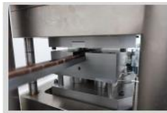
Specimen cross section (15.6 x 3.8) mm 2
