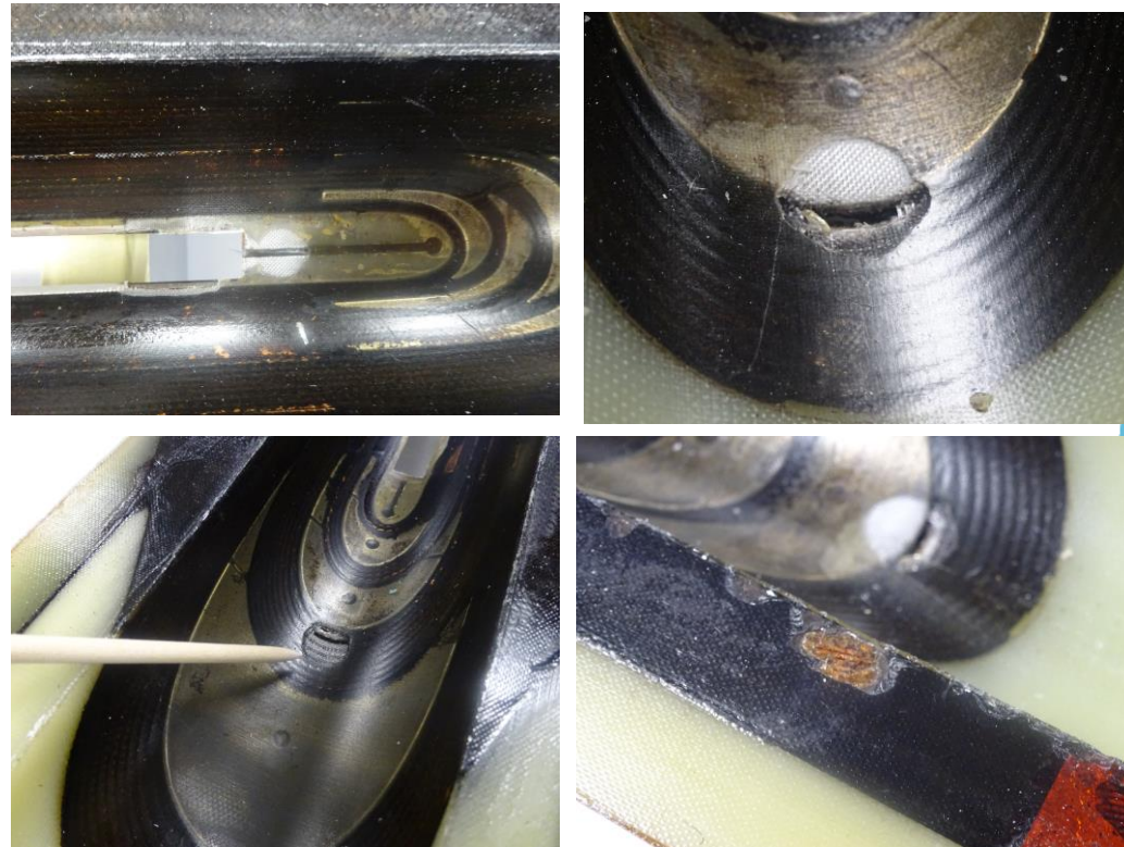
Coil 114, coils with quite big defaults after impregnation which were repaired*
