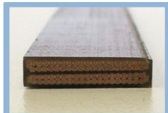
Specimen cross section (15.6 x 3.8) mm 2
