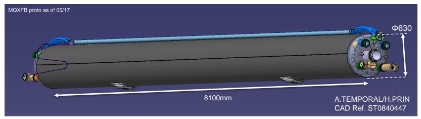
In order to provide a suitable cryostat for this activity it was decided to **reuse and adapt a spare LHC MS Q4 cryostat** to fit the dimensions displayed above and provide an exit routing for the instrumentation.
