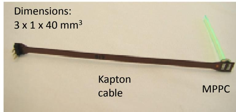
The **photodetectors** are Geiger mode Avalanche Photodiodes (G-APD = SiPM) of type MPPC from Hamamatsu.
