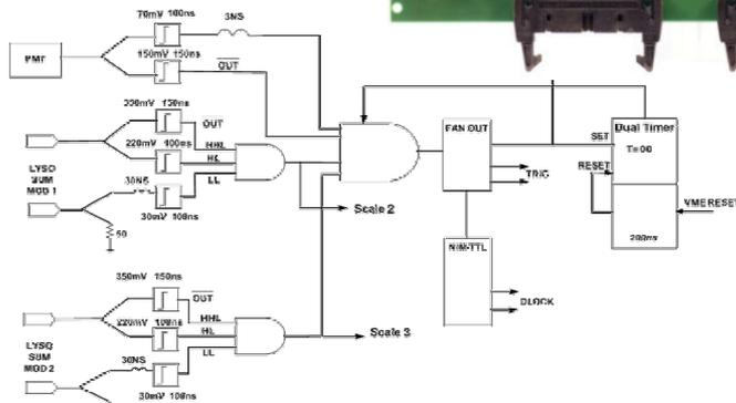
AX-PET Trigger Block Diagram
