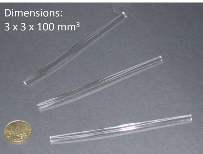
The **WLS strips** are of type EJ-280-10x from Eljen Technologies
