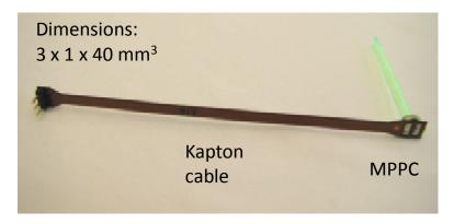
The **photodetectors** are Geiger mode Avalanche Photodiodes (G-APD = SiPM) of type MPPC from Hamamatsu.
