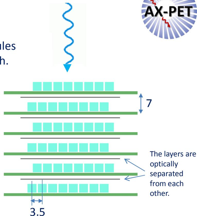
Crystals are staggered by 2 mm. Crystals and WLS strips are read out on alternate sides to allow maximum packing density.
