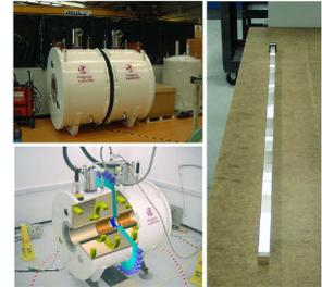
Fig. 4. (a) Split magnet design for combined PET/MRI. (b) The PET detectors will be located in the gap with the optical fibers emanating radially as shown. (c) View of (front) a single PET detector module with scintillator array connected to (back) a position-sensitive PMT by optical fibers. Adapted with permission from [23].
