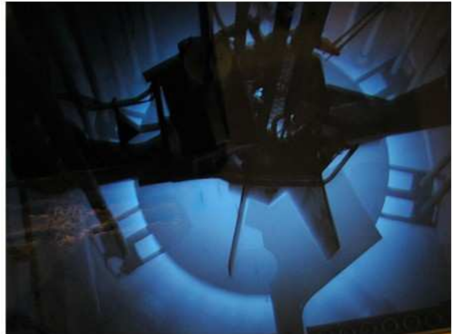
Blue "Cerenkov radiation" from MAPLE 1 reactor core during commissioning tests at high power (8 MW). The Cerenkov glow is caused by high-speed electrons (beta particles or secondary electrons due to the core's operation) slowing down in the surrounding water.
