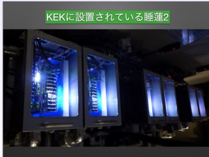
**Figure:** Suiren2 at KEK, liquid immersion cooling, many-core supercomputer
