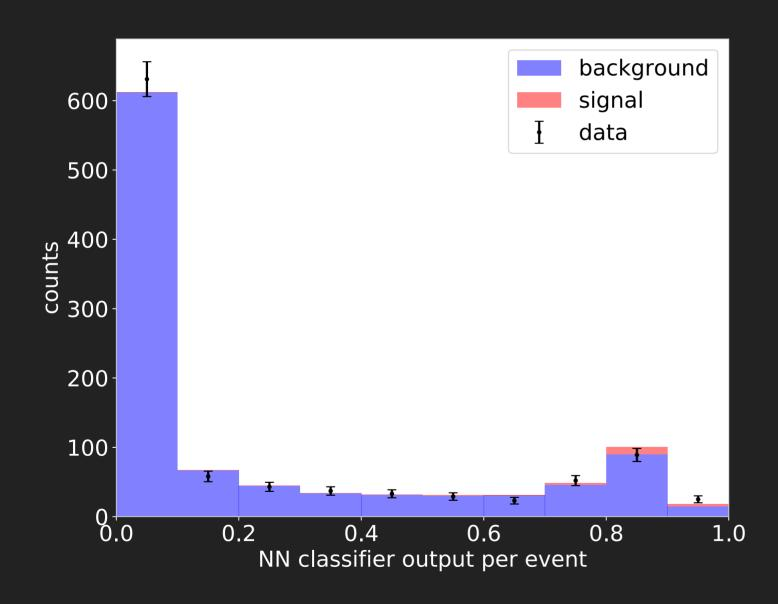
1-D → cut or histogram to build a Poisson counts non-parametric likelihood
