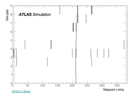
Example of a muon with  $p_T$ =19 GeV + noise
