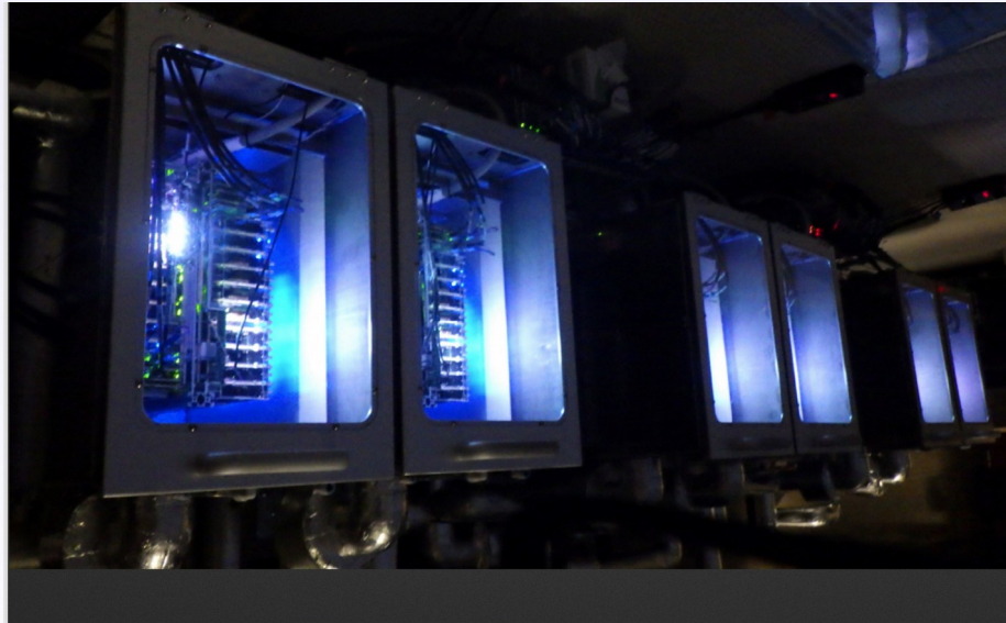
Suiren2 at KEK, liquid immersion cooling, many-core supercomputer
