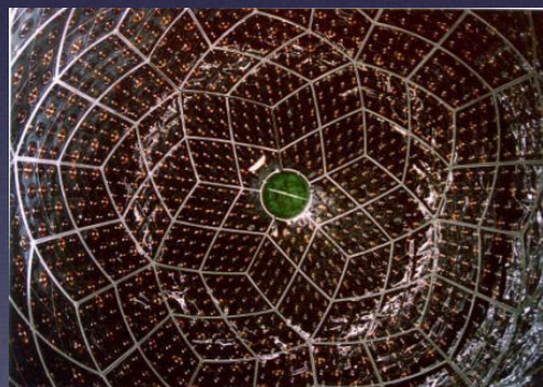
Liquid Scintillator 1 kton, 1900 PMTs (2002)
