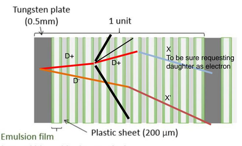
(50 μm thick emulsion layers on both sides of a 200 μm thick plastic base)
