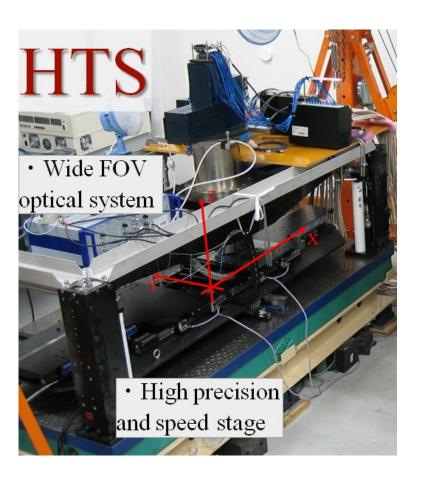
Scanning system working at Nagoya Univ, scanning speed of 9000 cm<sup>2</sup>/h (22 m<sup>2</sup>/day)
