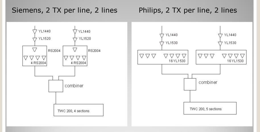
Total voltage (2 cavities): 4.1 MV w/o BL, Total voltage (2 cavities): 5.5 MV w/o BL,  $\approx$  3.3 MV with nominal BL (1.15 10<sup>11</sup> ppb). With new tubes: 350 kW/TX
