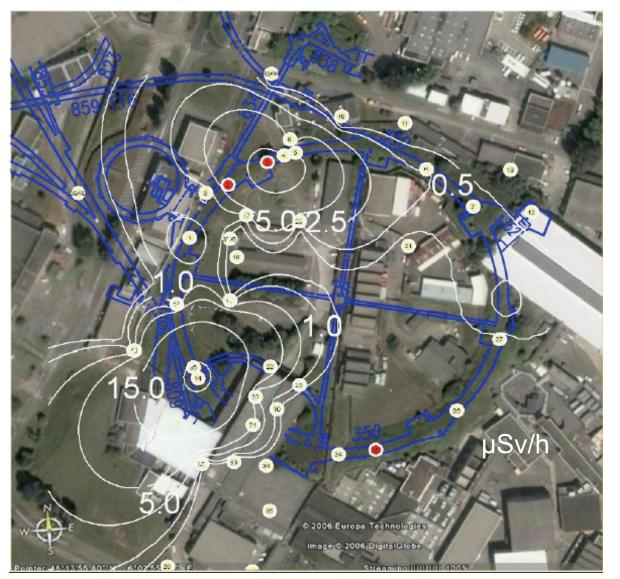
2007 radiation survey outside the PS tunnel during CNGS operation at about 0.8 p/s.
