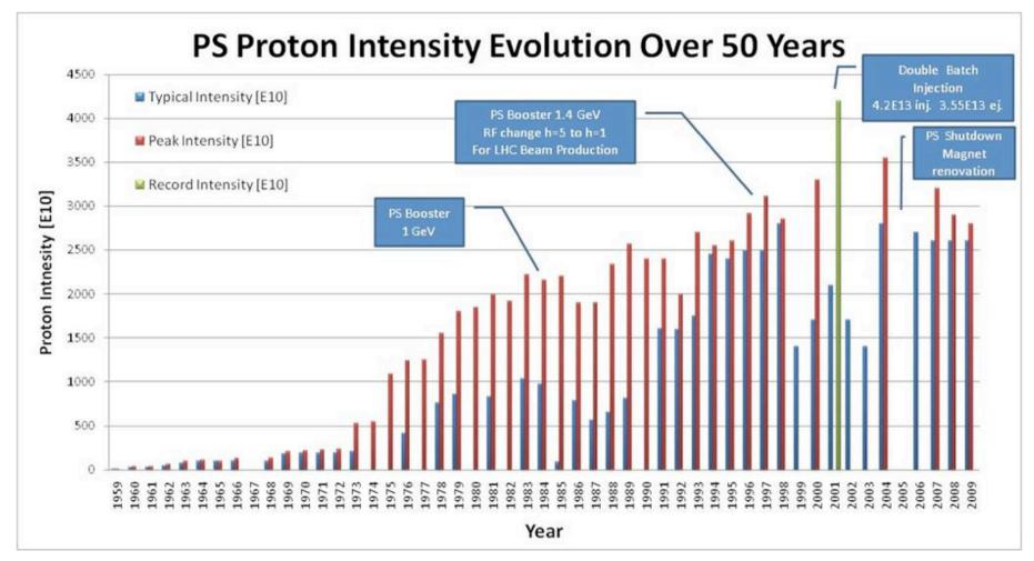
Increase of machine irradiation is not produced by an increase of the maximum intensity but by the high repetition rate required by the CNGS operation.
