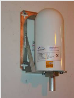
Gas filled, high pressure ionisation chamber
