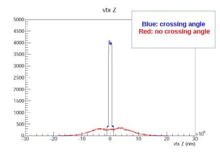
Plot showing the Z coordinate of the vertex of beam particles that interact to produce an  $e^+e^-$  pair for  $E_{cm} = 91.2$  GeV. The 2 histos are not in scale
