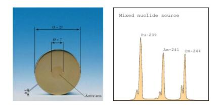
Mixed  $\alpha$ -source (Pu, Am, Cm) shooting through 7 mm hole in the cathode Rate ~550 Hz
