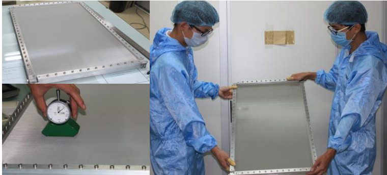
Mesh stretching \sim 20\text{N/cm}
