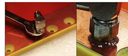
Figure 12: Fixing the gas connector onto the board.
