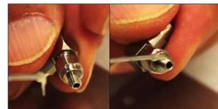
Figure 11: Applying glue to the gas connector.
