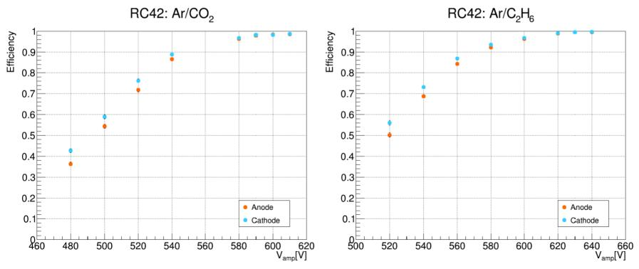
More than 98% of efficiency is obtained using both Ar/CO2 gas and Ar/C2H6 gas
