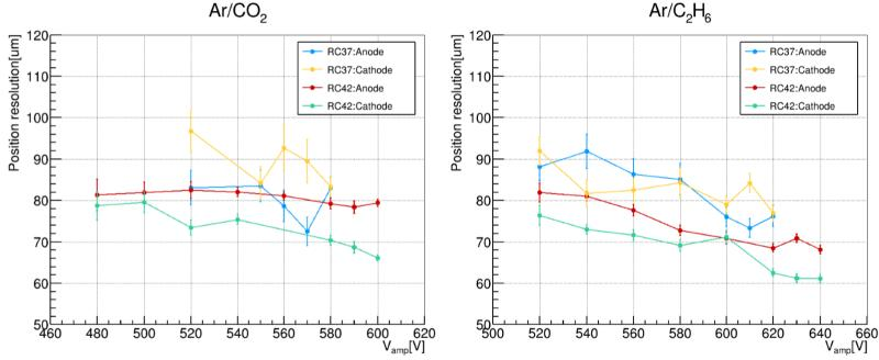
Less than 70um of position resolution are attained on two dimensional readout using Ar/C2H6 gas
