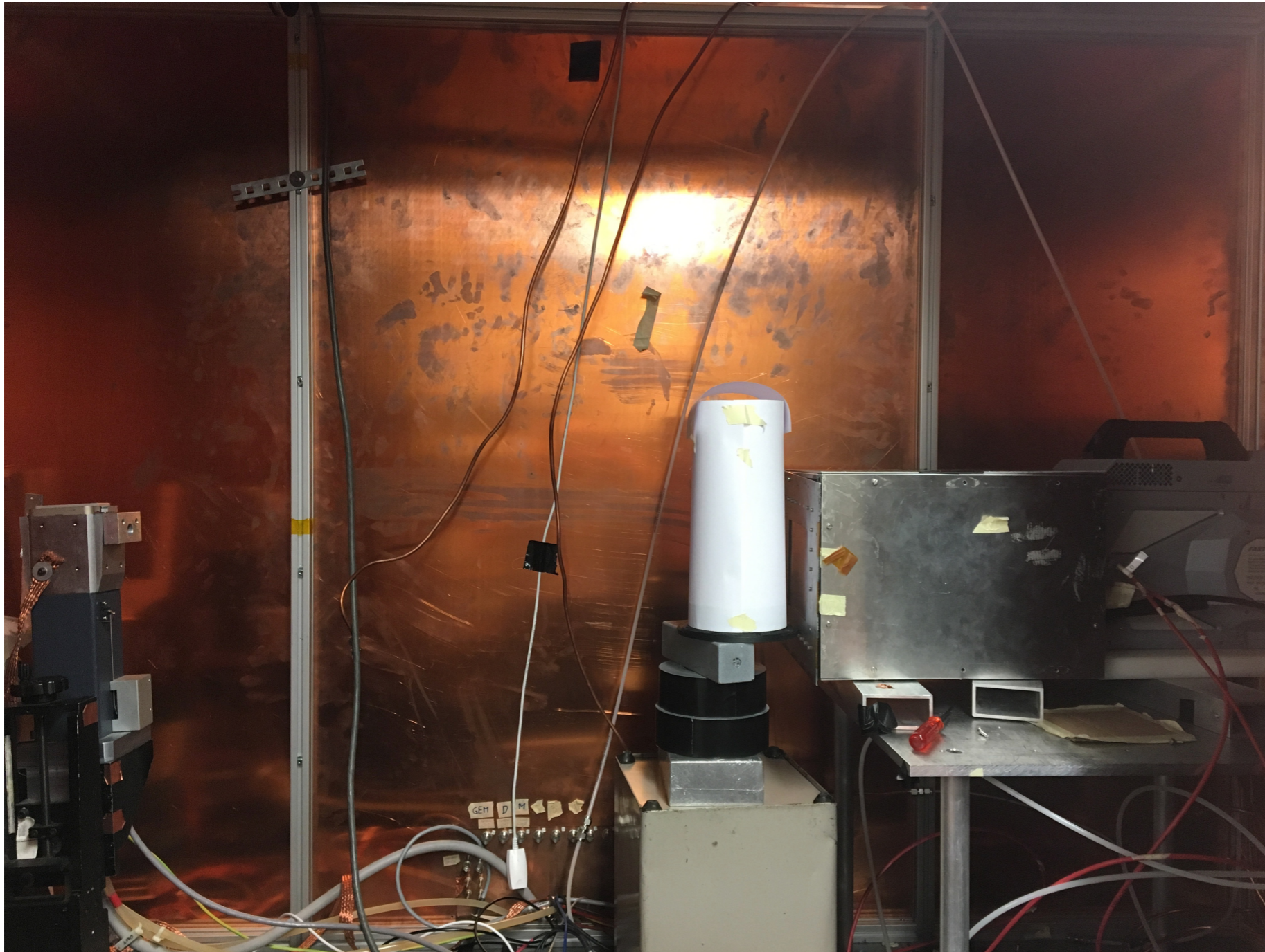
Remote controlled Blade drone in paper cylinder in front of detector irradiated with X-ray tube
