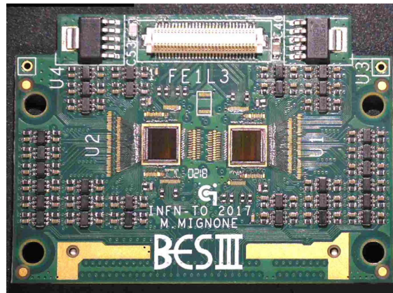
2 TIGER ASICs wire-bonded on the Front-End Board (FEB)
