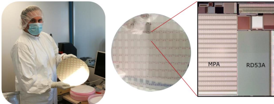
First 12" wafers at CERN with RD53A
