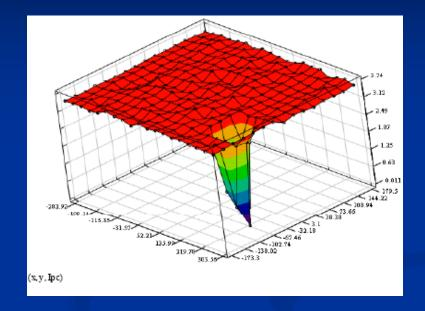
• Quantum efficiency segmentation on the photo cathode level
