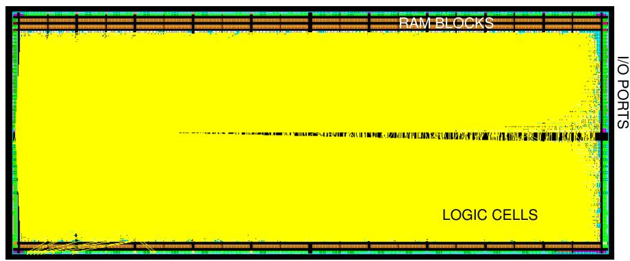
Core used: 96.3% (of 38400 cells) in this simplest configuration.
