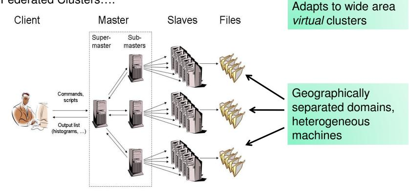
Super master is users' single point of entry. System complexity is hidden Automatic data discovery and job matching with local data
