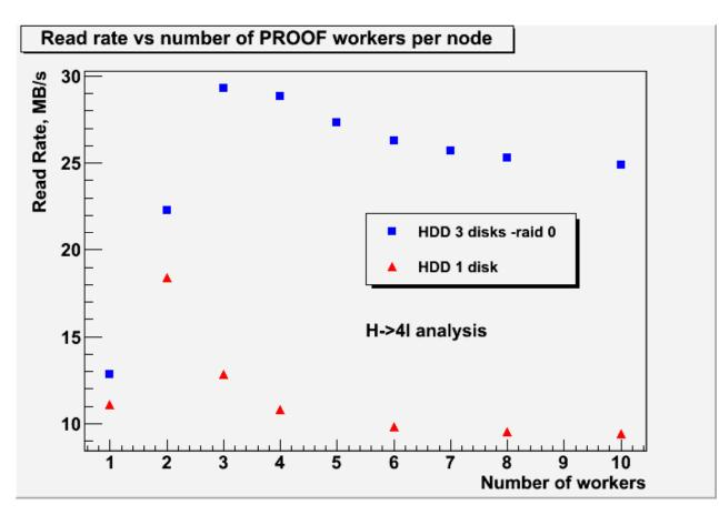
3x750 GB HDD RAID peaks at ~3 worker load Single HDD disk peaks at 2 worker load, then performance rapidly deteriorates
