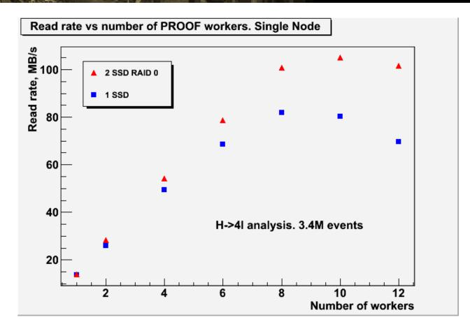
SSD 2 disk RAID 0 shows little impact up to 4 worker load
