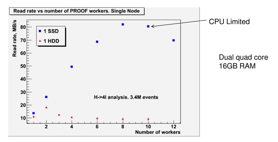
SSD is about 10 times faster at full load Best HDD performance at 2 worker load Single analysis job generates ~10 -14 MB/s load with given hardware Sergey Panitkin
