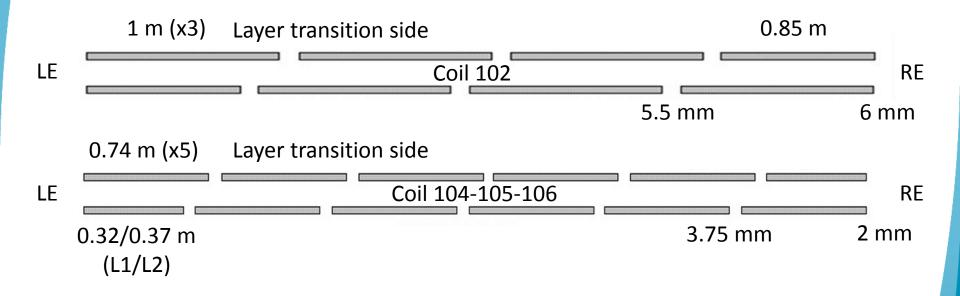
Axon (CERN recommended vendor) wires utilized for protection heaters and voltage taps in coils 104, 105 and 106.
