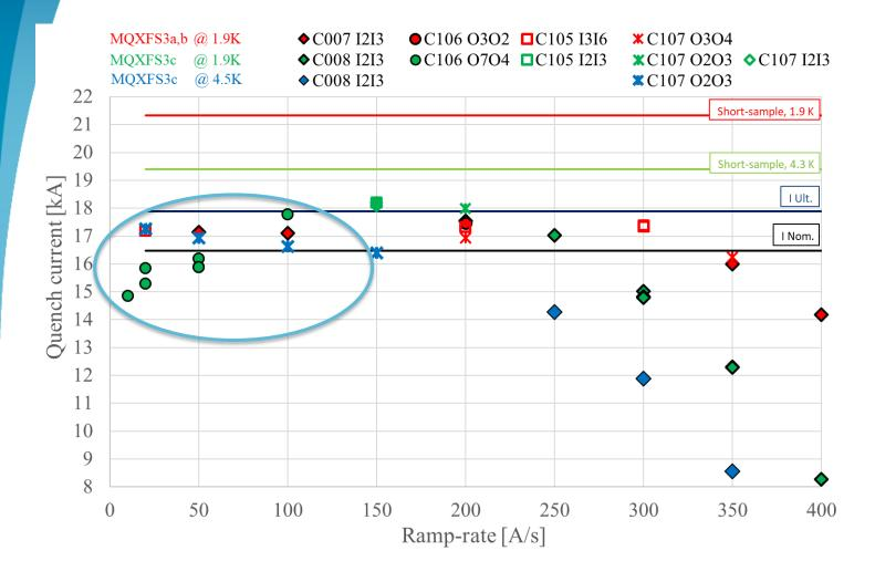
The comparison with the results obtained at 1.9 K confirms "the self-field instability enhanced by a damage in Coil 106" Unlike 1.9 K behaviour, the quench current at 4.5 K decreases with the ramp rate.
