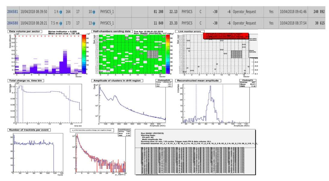
to measure  $v_{drift}$ . Fast reconstruction is going on now. 73 FEDs disabled due to HV anode channels off, in addition to 22 from last year.
