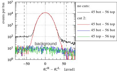
Trigger: double-arm RP RP tracks in opposite arm in diagonal topology Cuts: left-right correlation in several kinematic variables
